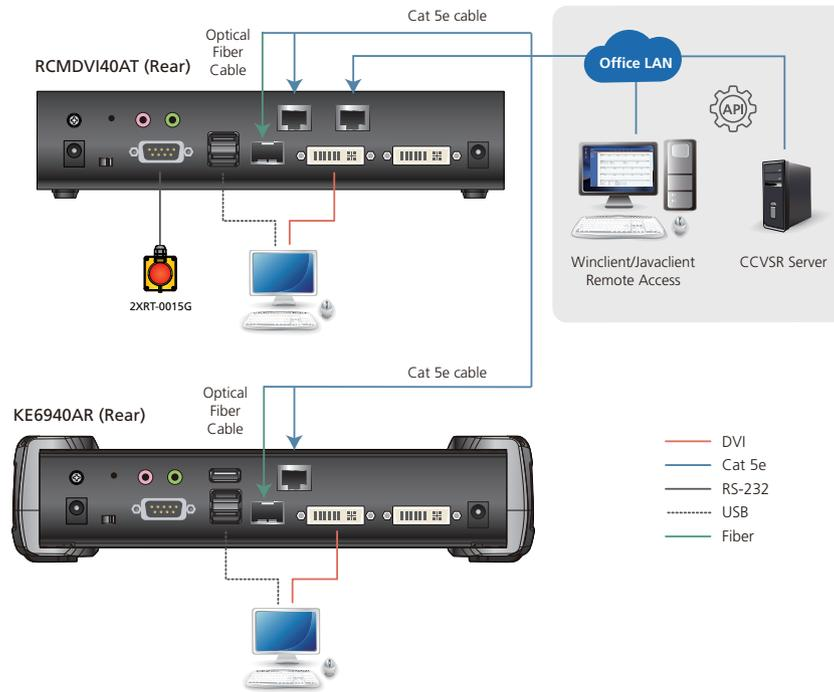
**RCMDVI40AT Matrix Mode Reference Installation Diagram**
